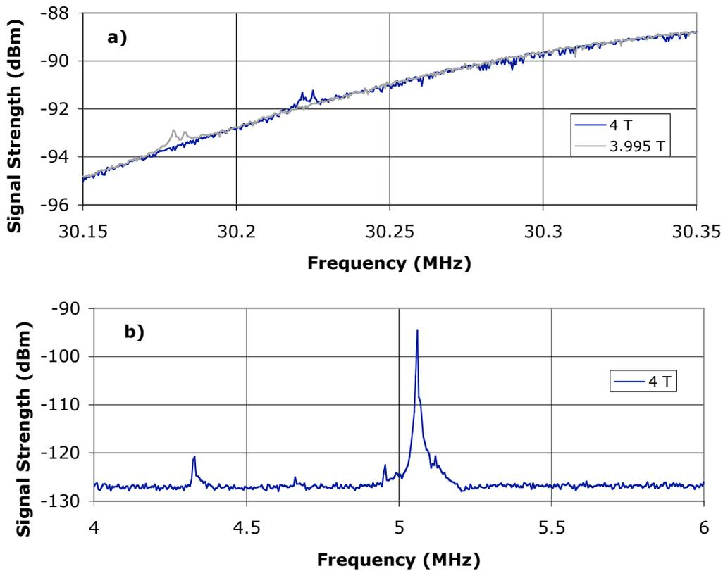
FIGURE 5. a)  $\omega_+$  at Two Magnetic Field Strengths for  $H_2^+$  Ions; b)  $\omega_+$  for  $C^+$  Ions.
