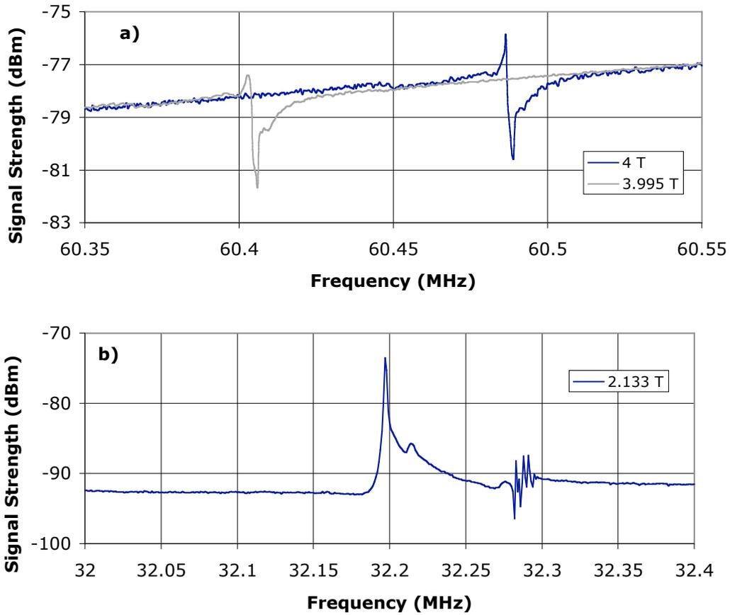
FIGURE 4. Change in Modified Cyclotron Frequency With Change in Magnetic Field Strength
