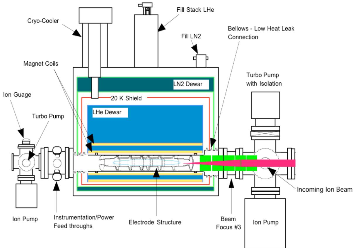
FIGURE 1. Layout of the HiPAT Experiment.
