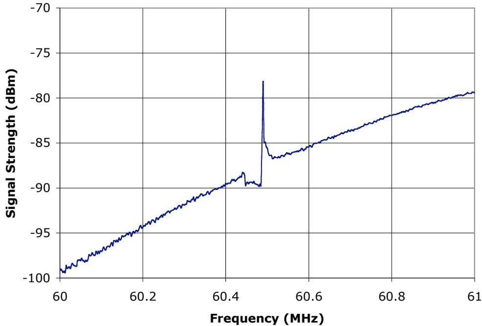
FIGURE 3. H<sup>+</sup> Cyclotron Signal After Injection on Day 1.
