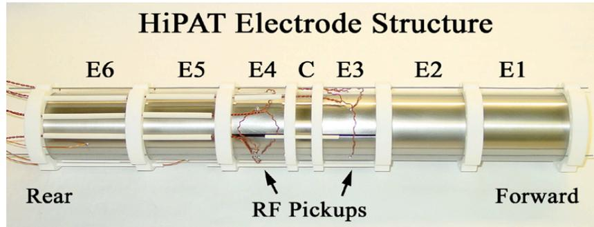
**FIGURE 2.** Electrode Structure Inside HiPAT (E3 and E4 are Made of Four 90° Azimuthal Segments).
