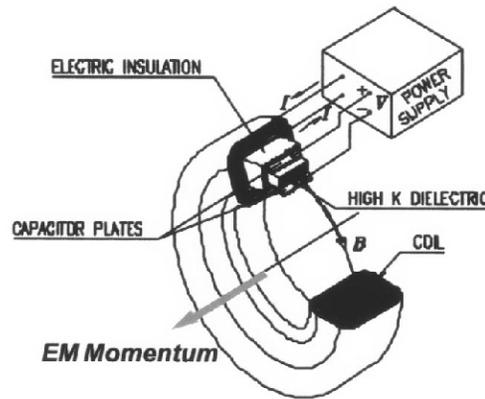
**FIGURE 2.** H. Brito’s Schematic Diagram of his “Electromagnetic Stress Tensor” Device.
