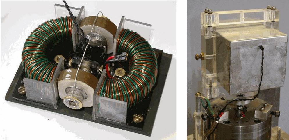
(a) A Hybrid Mach-Slepian Device with High Voltage Capacitors Mounted Between High Flux Inductors.
