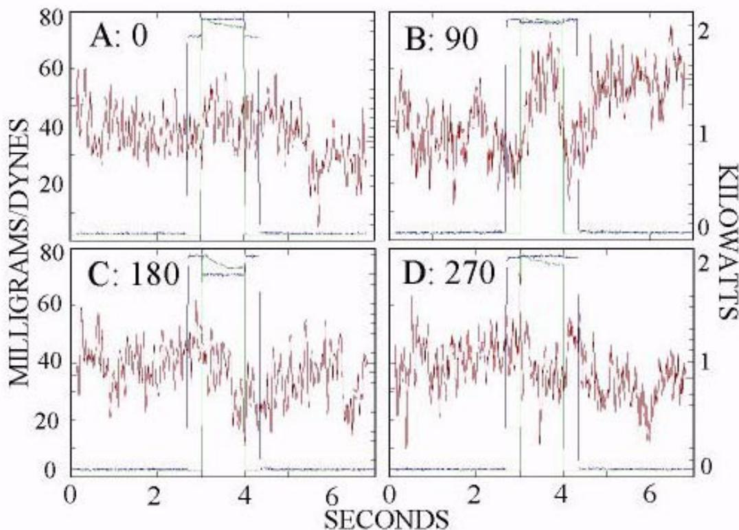
**FIGURE 4.** The Thrusts Measured with Mach 3 at the Indicated Relative Phases for the Voltage in the Capacitors and the Current in the Inductors.
