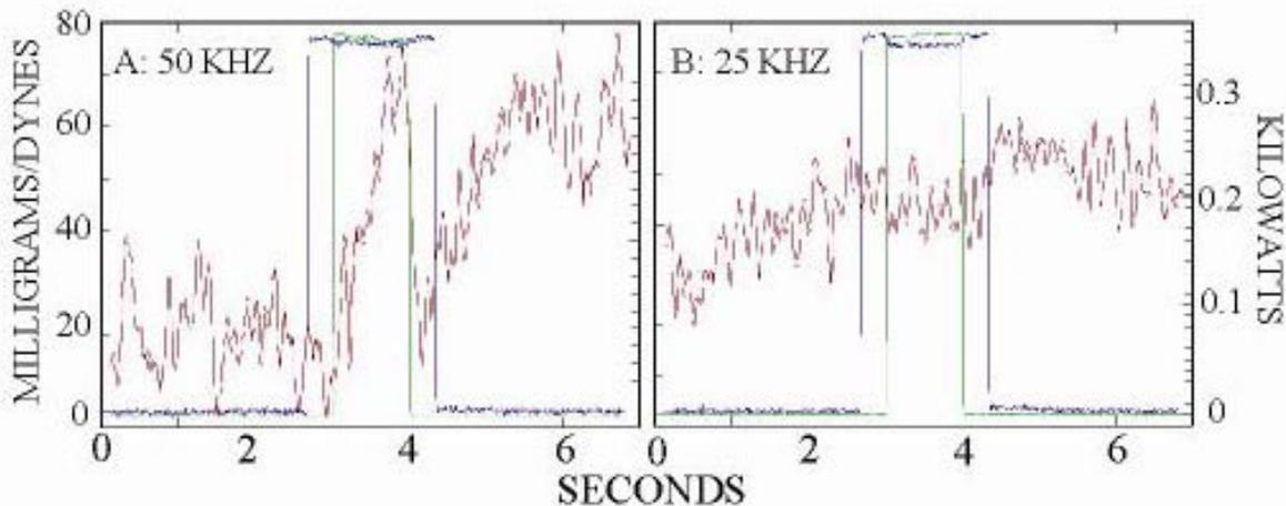
**FIGURE 5.** The Thrust Responses at 50 and 25 kHz. (The 25 kHz Data are Consistent with the Mach-Slepian Scheme. They are not Consistent with the Purely Electromagnetic Scheme.)
