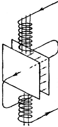
**FIGURE 1.** A Schematic Diagram of a “Slepian” Inductive-Capacitive Circuit (after Corum, *et al.*, 1999).
