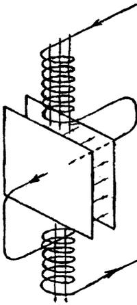
Fig. 2. A schematic diagram of a “flux” capacitor [after Corum, *et al.*<sup>(14)</sup>] in which the material between the plates of the capacitor is subjected to an AC electric field and a perpendicular, high flux AC magnetic field produced by the inductors ranged above and below the capacitor in the drawing.
