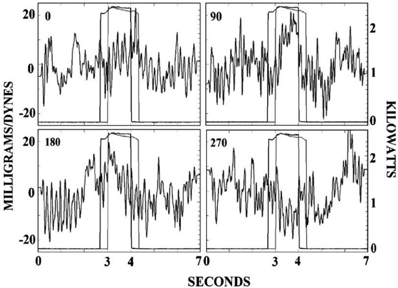
Fig. 7. Results (averages of about 200 cycles) for the four relative phase angles between the inductor current and capacitor voltage at high power (roughly 2.5kW amplitude power wave delivered to the capacitors).
