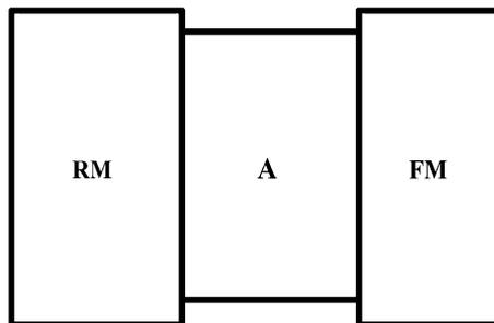
Fig. 1. A schematic diagram of a Mach effect “impulse engine” comprised of a reaction mass (RM), piezoelectric actuator (A), and a fluctuating mass (FM) element in which the Mach effect is driven.
